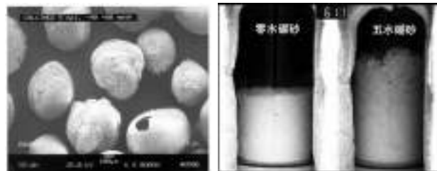
Figure 4. volume change during the heating process. (a): expanded spheres of borax pentahydrate during dehydration; (b): comparison of batch volumes. Each batch contains 5% \text{B}_2\text{O}_3 . Left crucible is a batch containing Dehybor® and right crucible is a batch containing borax pentahydrate. Temperature recorded was 611°C
