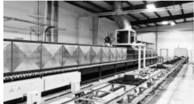
Cooling section of a roller furnace for cast iron pots
